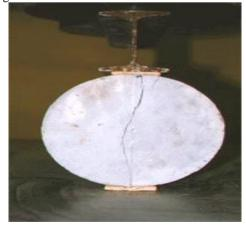
The Brazilians test namely gives consistent results that lie between those based on other two methods (wrigh-1955). In this method the split tensile strength,
