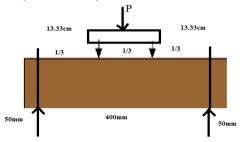
The modulus of rupture is determined by the formula,  $f_r = \frac{M}{bd^2} = \frac{PL}{bd^2}$
